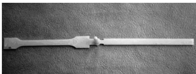
Figure 1 Schematic diagram of the injection-molded bars for mechanical test. (Left, bar for tensile test; Right, bar for impact test).
