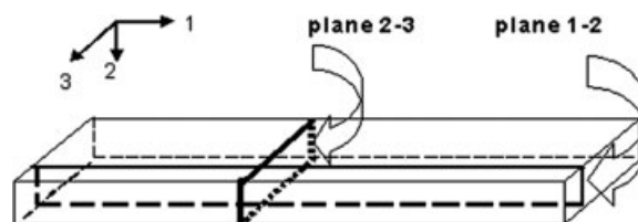
Figure 2 Schematic diagram of the fractured surfaces. (1 is the direction of flow, 2 the thickness direction, and 3 the transverse-wide direction).
